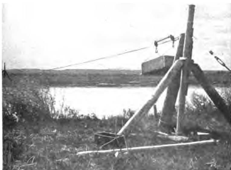
FIG. 52.—Cable and Car Gaging Station.
